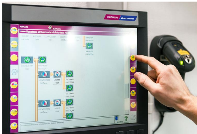
WITTMANN M7.3 IPC touch-screen network control system. On the right, a barcode scanner is mounted on the wall. The control system monitors the material flow from the material source to the processing machine.
