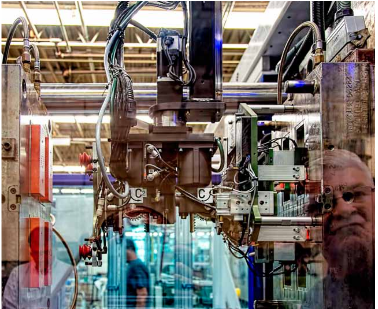
WITTMANN W833 robot with specially designed EOAT, places metal inserts and removes finished parts in the same in/out cycle.
