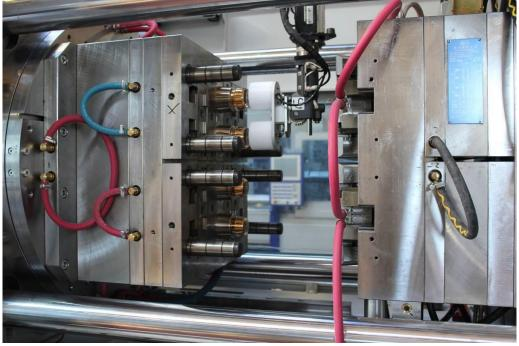
Fig. 2: Mold for the production of cream jars in 2-color technology
