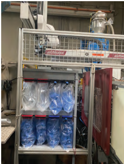
The WITTMANN PRIMUS robot separates cavities, counts and packs dental parts into bags for shipping.
