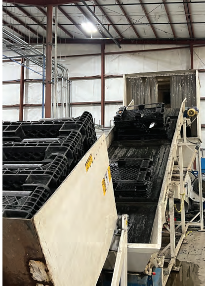
Scrap totes on conveyor on their way to granulator for grinding
