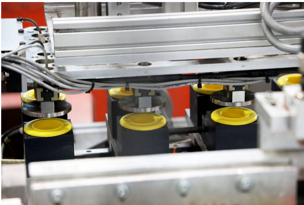
Fig. 3: WITTMANN gripper picking up the wheel rims
