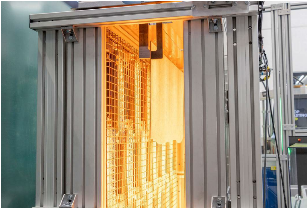
Fig. 2: Heating of the pre-cut natural fiber mat in IR heating station
