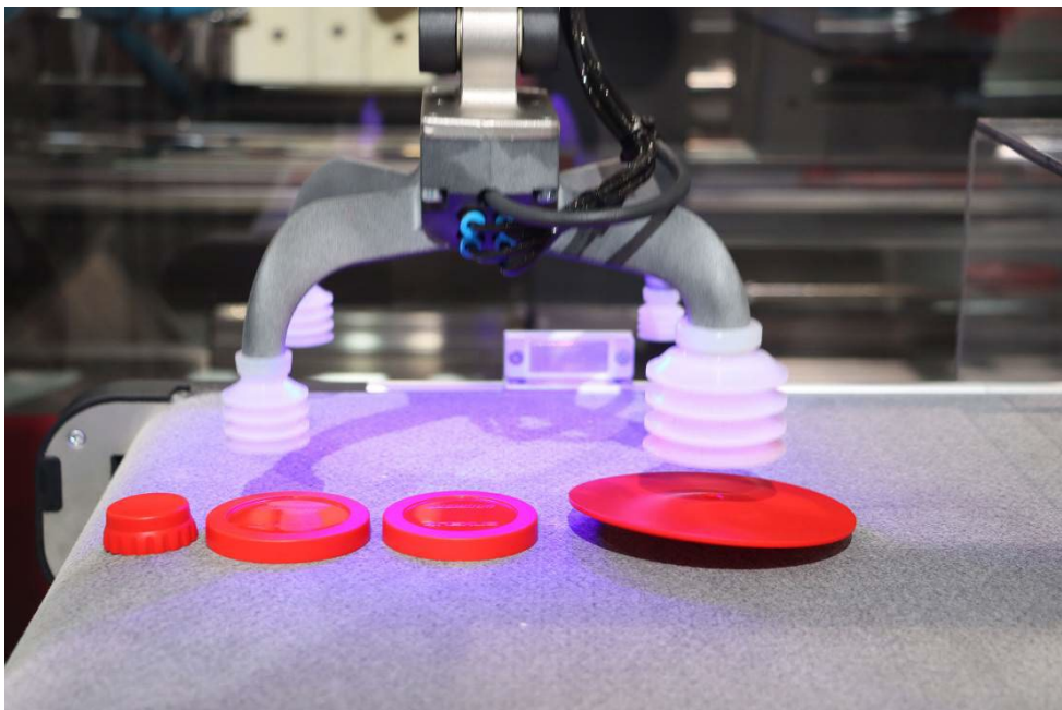
Fig. 2: LSR closing caps for beverage cans
