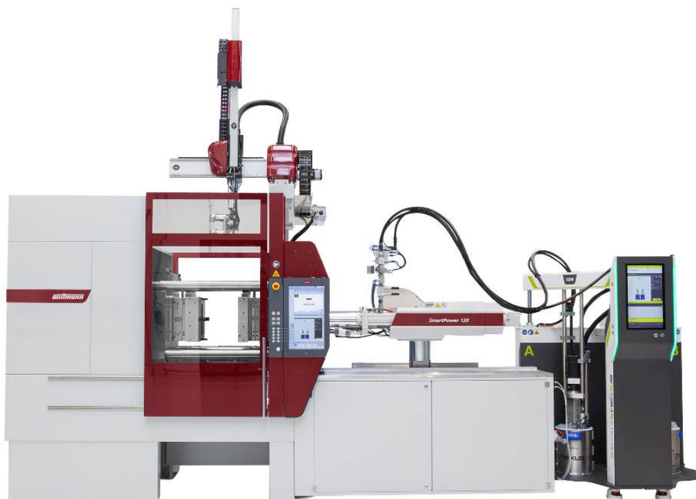
Fig. 4: SmartPower 120/350 LSR with Nexus X200 dosing unit
