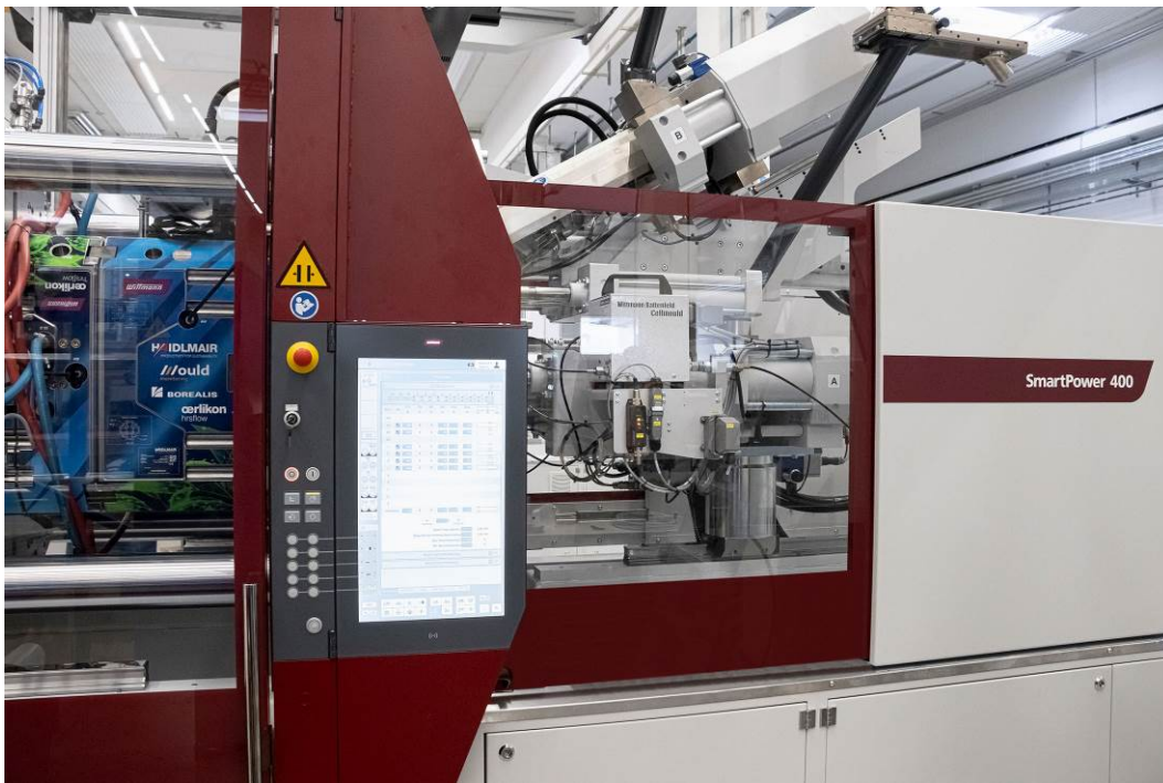
Fig. 1: SmartPower in 3-component version equipped with Cellmould technology
