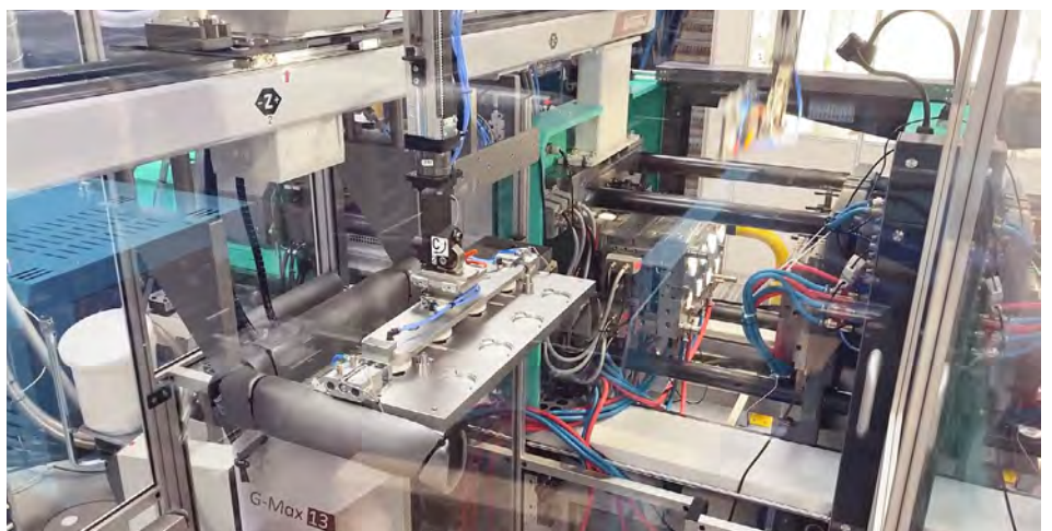
The removal robot moves back into the mold area of the injection molding machine, while the other robot again picks up the parts from the transfer station.
