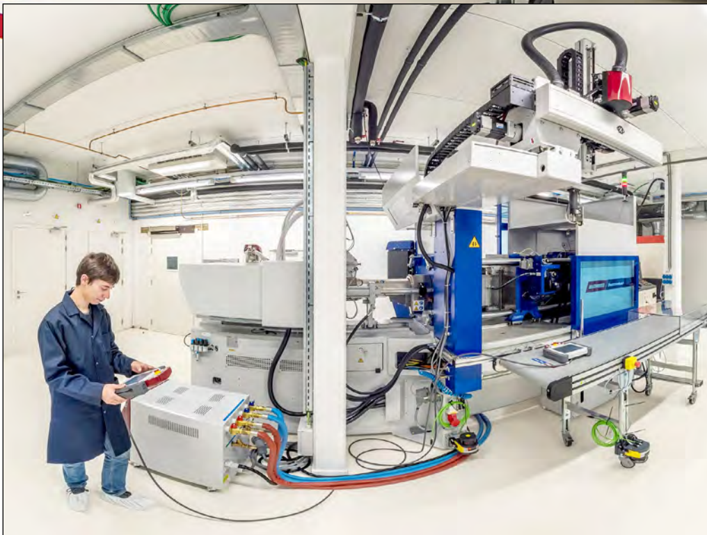
Views of the EcoPower production cell supplied by WITTMANN BATTENFELD Benelux NV at the B-PHOT research department of the Vrije Universiteit Brussel with W818 robot, variothermal Tempro plus D180 temperature controller, and Aton plus VS segmented wheel dryer with material conveying. All devices are connected to the molding machine via Wittmann 4.0.
