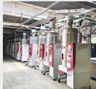
Page 8: The new central conveying system of Husqvarna (CZ).
