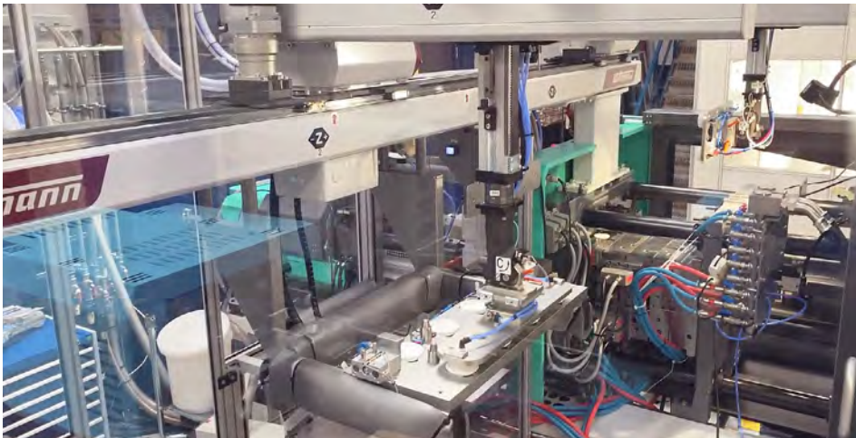
While the second robot places the parts on a conveyor belt, the removal robot positions the removed parts on the transfer station.
