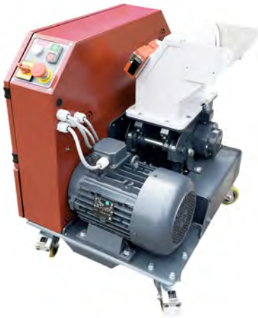
G-Max 9 granulator installed under the injection molding machine in the clean room.
