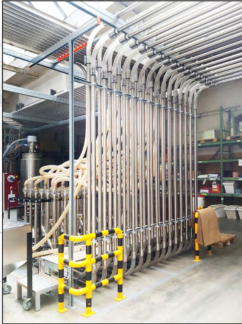
Two examples of the integration of peripheral equipment from different manufacturers: conveyors with control components from WITTMANN (left) and WITTMANN material dryers, each with different conveyors on the drying hoppers.
