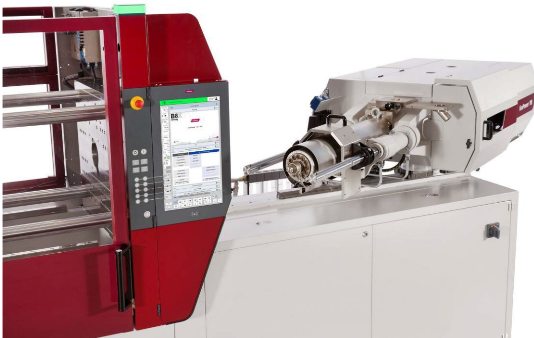
Fig. 2: Pivoting injection unit
