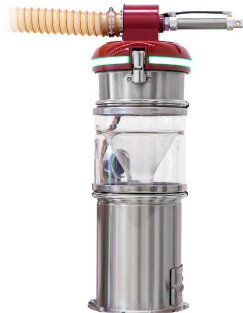
Fig. 6: Feedmax Clean conveyor with dedusting function
